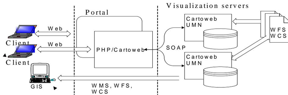
Fig. 4. Visualization system using thick client
